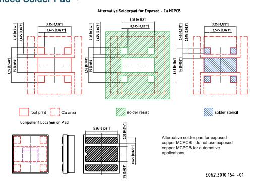
Exposed Copper MCPCB must not exceed thickness of 1mm. For superior solder joint connectivity results we recommend soldering under standard nitrogen atmosphere. Package not suitable for any kind of wet cleaning or ultrasonic cleaning.
